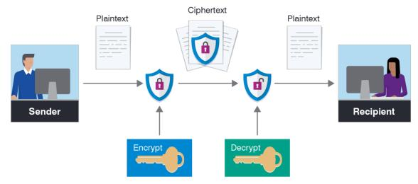
Different keys are used to encrypt and decrypt messages
